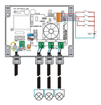
Given above is an example wiring for the 4 external control input signals. The table below describes the functions of the 8 pins of the external input connector.
