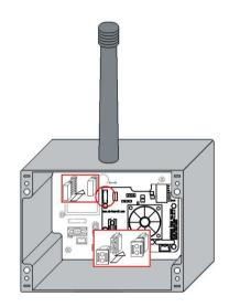
After the light control board is mounted on top of the Range extender / Accesspoint board, connect the input power connector of the light control board into the socket on the range extender/accesspoint board.
