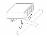
Place each of the double sided adhesive strips on one of the slanting V sides on the bottom part of the Xtra.shutdown transponder.
