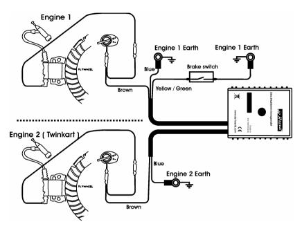
Depending on the type of Xtra.Shutdown transponder you use, one or 2 cables are coming out of the Shutdown transponder. The second cable on an Xtra.Twin Shutdown transponder is connected in a simular fashion as the cable for the first engine, and therefore not specifically described in the text below.
