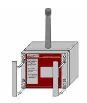
Lift the plastic design covers of the Xtra.RangeExtender-Accesspoint from the aluminium housing.
