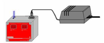
Push the adapter power plug completely into the socket on the Xtra.Sector Beacon. Once the plug is put correctly into the socket, fasten the plug with its locking screw. Once locked, the connection is water resistant.
