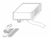
By means of 2 tiewraps and 2 double sided adhesive strips it is possible to mount the Xtra.Shutdown transponder in most cases.
